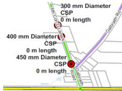
Figure 3: Middleville culvert locations and diameters
