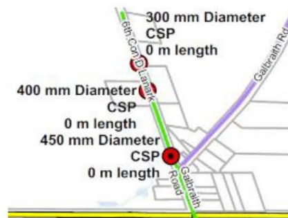
Figure 3: Middleville culvert locations and diameters
